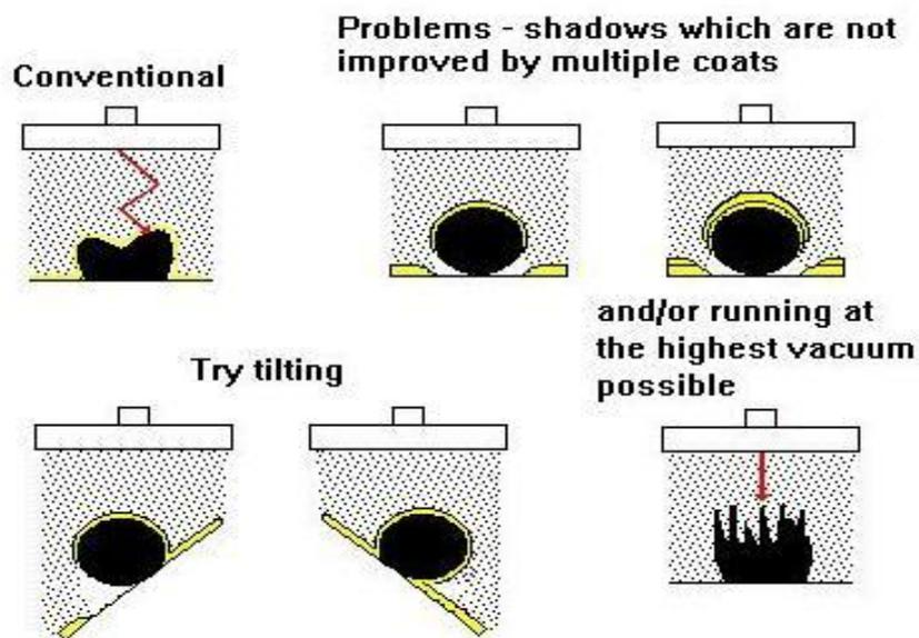
Tooth brush shaped specimens may also need a "straight line" coat by running the system with the gas turned off. Leakage is usually enough to enable you to strike a plasma but a higher than normal voltage will be required.
