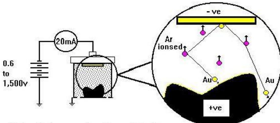
Modern Coaters use a deposition control or the gas flow to adjust the current at a low sputtering voltage. Older style coaters use a higher sputtering voltage the current being controlled by a voltage regulator or the gas flow.
