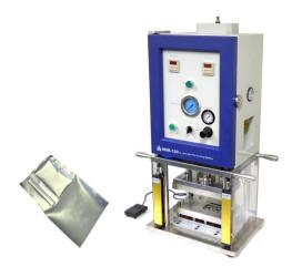
MSK-120 is a forming machine to prepare various cup-shape pouch cell cases from aluminum laminated film up to 250 mm x 200 mm in area and 6.0 mm in depth. It is a necessary tool for making polymer Li-Ion battery.
