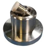
3. The old crimping head can now be swapped out and replaced with a new one. Ensure the new unit is aligned and seated properly and then tighten the crimping head holder with hand.
