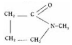
**Characteristics:** Transparent liquid, boiling point  $204^{\circ}$ C, flash point  $91^{\circ}$ C, strong moisture absorbability, amalgamate with water and diethyl ether, acetone and all sorts of organic dissolvent.
