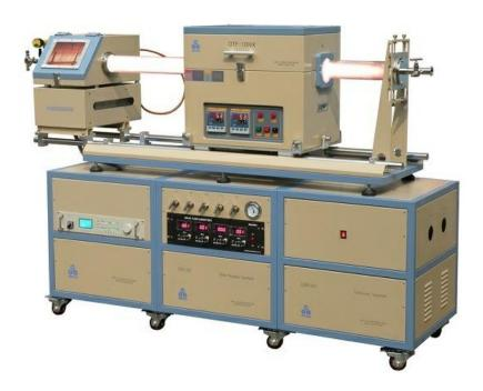
OTF-1200X-80-II-4CV-PE-SL is a dual zone slidable PE-CVD tube furnace system consists of 500W RF plasma source, 80Dx1600L mm split tube furnace with an integrated slidable rail, a 4-channel precision mass flow meter with gas mixing tank, and a high quality oil-less vacuum pump. Such a PE-CVD furnace is a new tool to grow Nano-wire or graphene with the following benefits:
