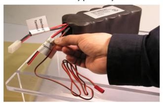
2. Connect the Chun-180 charger (Multi current universal smart charger for 9.6v-18v Nimh/Nicd battery pack) with the connector adaptor provided. (Standard Tmaiya Male end of the connector adaptor connect to Standard Tamiya Female plug of the charger)
