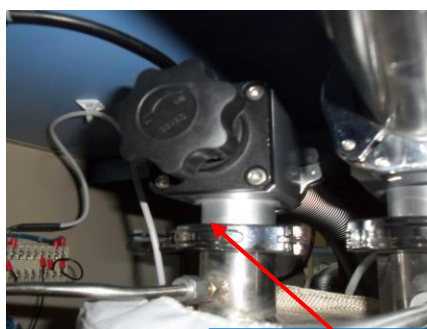
Open the Right Angle Valves 1 & 2, Circulation path OPEN
