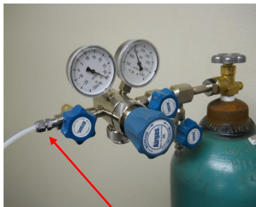
Connect other side to high purity Nitrogen Gas
