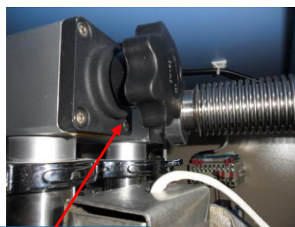
Open the Right Angle Valves 1 & 2, Circulation path OPEN
