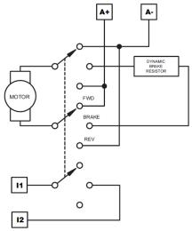
Figure 18. Reversing Circuit Connection
