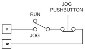
Figure 16. RUN/JOG Switch Connection to I1 and I2 (Option #1)
