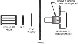
Figure 3. Speed Adjust Potentiometer
