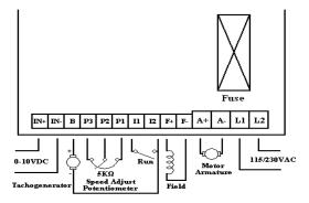
Figure 6. BC11 Connections
