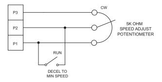
Figure 11. Run/Decelerate to Minimum Speed Switch
