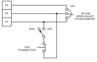
Figure 17. RUN/JOG Switch Connection to Speed Adjust Potentiometer (Option #2)
