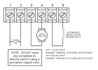
Figure 9. Cased Drive Connections
