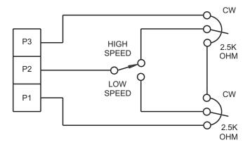
Figure 14. Adjustable Fixed Speeds Using Potentiometers in Series
