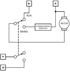
Figure 12. Dynamic Brake Connection
