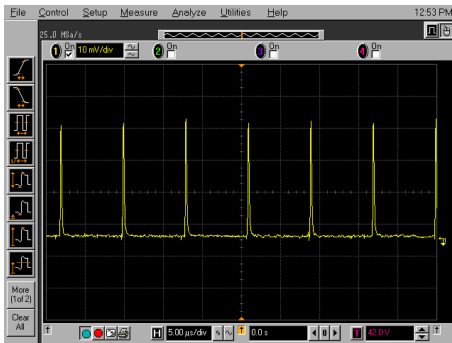
Fig. 8. Pulsed 532nm output generated by the intracavity-doubled of VECSEL (1064nm) laser.
